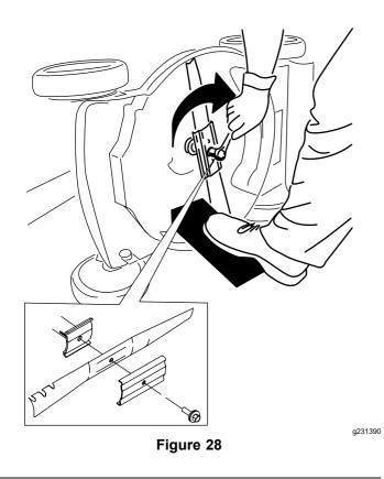
Important: Position the curved ends of the blade to point toward the machine housing.
