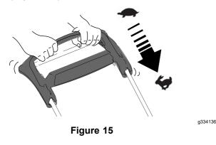
**Note:** If the machine does not freely roll backward after self-propelling, stop walking, hold your hands in place, and allow the machine to roll a couple of centimeters (inches) forward to disengage the wheel drive. You can also try reaching just under the upper handle to the metal handle and pushing the machine forward a couple of centimeters (inches). If the machine still does not roll backward easily, contact an Authorized Service Dealer.
